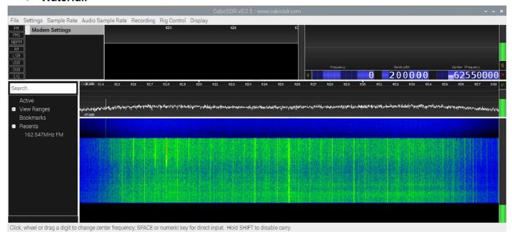
The frequency is on the upper right hand side. You can set this to a local radio station. In this example, we have set it to 97.300.000 with a bandwidth of 200.000. This relates to 97.3 on the radio dial. If you want to listen to 100.7, then you would set the numbers to 100.700.000. Once you set the frequency, the waterfall (center bottom) and the bandwidth view (upper left) should show you a bright orange and red stream of data.
